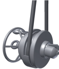
Turn the handwheel to open the clutch.
