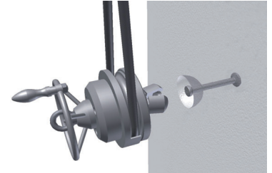
Press tightly onto the anchor head.
